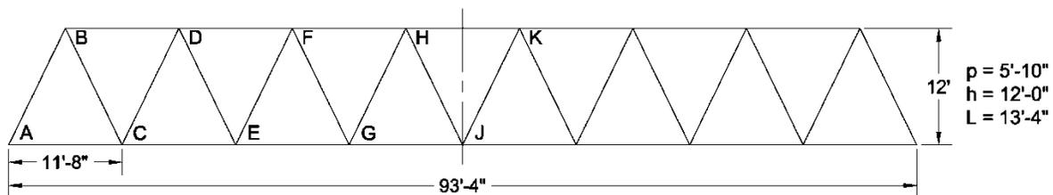
Figure 17: Truss Layout
