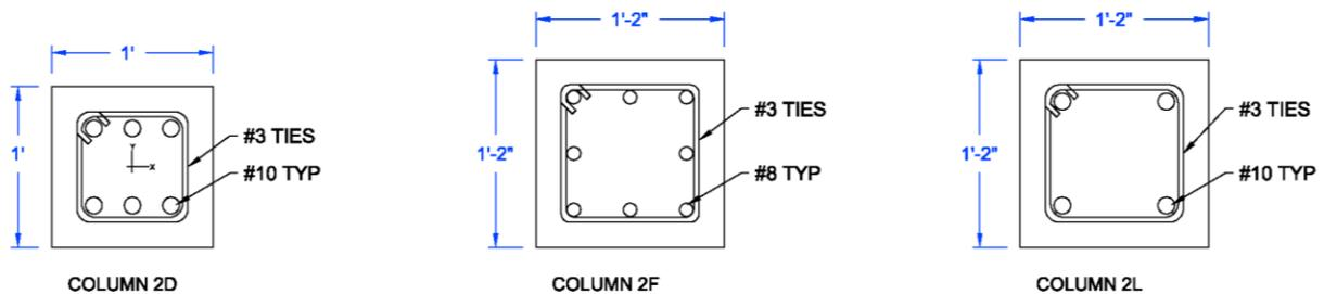
Figure 12: Column Designs for Column Line 2
