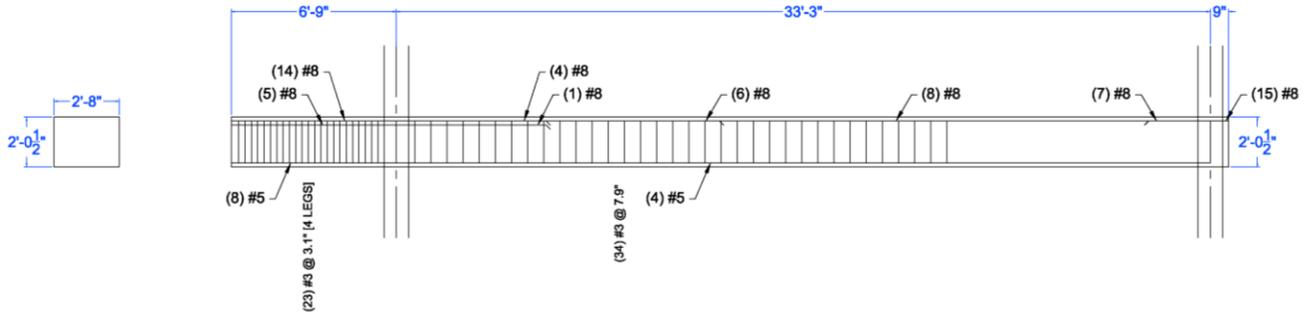
Figure 11: Beam Design for Column Line D
