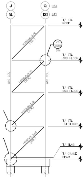
Figure 7: Typical Braced Frame
